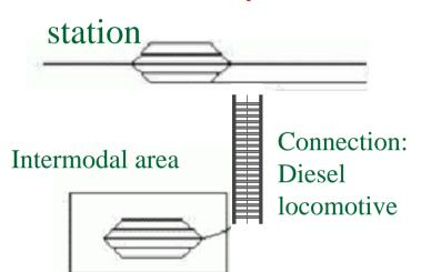
Today intermodal terminals are off-line. Trains must be shunted away from the electrified track using diesel locomotives, pulled to a loading yard, loaded, and brought back to the regular track by diesel traction. This operation usually takes 10–12 hours, with significant shunting costs (up to 70/100 euro per unit)
