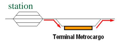
With Metrocargo® the loading unloading activity takes about 60 minutes. The trains remain under the electrical track and automatic handling permits the safety movements of containers.
