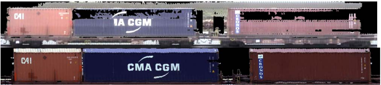
Figure 1 – Comparison between CAM4 (top) and MEGA (bottom) on a rather difficult situation (bright sun and wind) speaks in favor of the Megapixel technology
